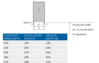
**TA** = seat engaging surface for gates. The dimensions must be agreed on site with the gate manufacturer.
